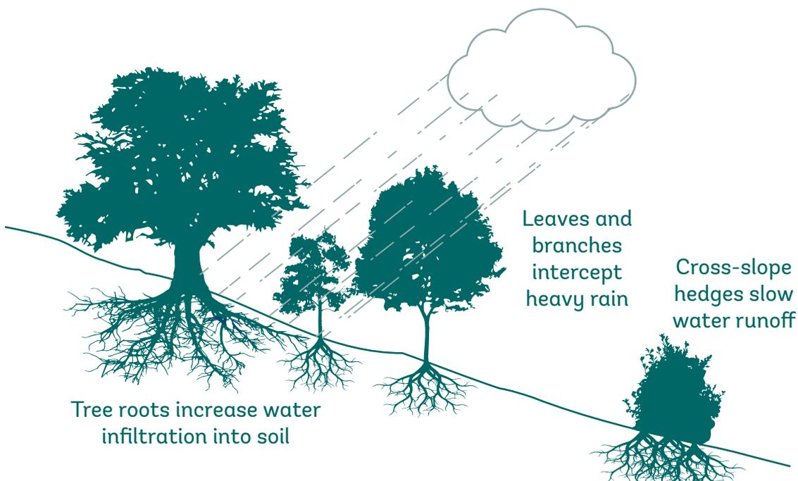
**Figure 4.10: Design to reduce surface-water flow**
