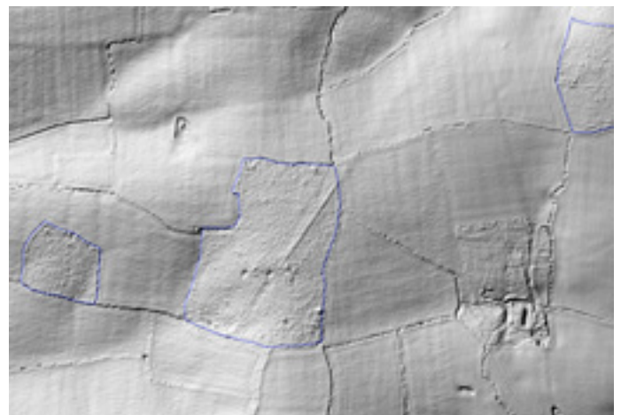
Brent Pelham LiDAR - Showing a strong lineal feature through an ancient woodland site, which is clearly less apparent outside the boundary. In this instance, the undisturbed soils within the ancient woodland have preserved the route of a Roman road.
