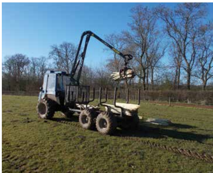
Unloading stakes and tubes with a forwarding machine due to waterlogged ground.
