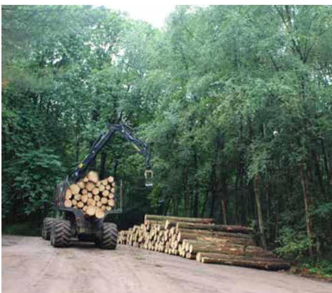
Good infrastructures of permanent tracks are important as part of restoration harvesting operations. Forwarder stacking timber at a loading area at an ancient woodland site in Surrey.
